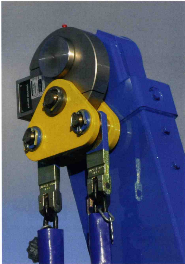
VWS's Skip Weigher uses a load cell on the top of lifting arm assembly
